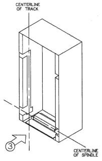
Step 3 – Center the Base Plate Spindle with the centerline of the track and press in place. You may need to rotate the Base Plate 180° for best alignment.
