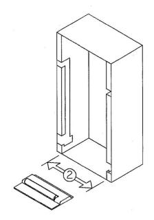
Step 2 – Center Base Plate between the dispenser sidewalls
